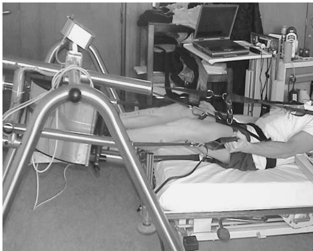
Fig. 1 The Galileo Space device used for resistive-like vibration exercise (RVE) protocols (RVE group) at supine position during 56 days of strict bed rest. During training, the bedridden candidate pushes the foot plantar region onto the vibrating Galileo platform ( left ) using elastic shoulder and hip straps and short elastic cords held in both hands (daily bouts 2×6 min at a.m./p.m.). During exercise, however, short but high repetition mechanical load (i.e., leg extension vs. acceleration) is transmitted alternately to each leg via the vibrating platform. We therefore defined this protocol RVE
